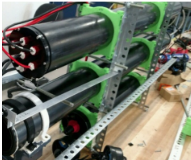
Figure 2:L-channel brackets design
